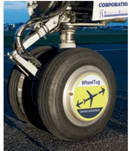
LEFT Honeywell and Safran's EGTS uses the auxiliary power unit to power motors on the main wheels. TOP The WheelTug system during ground testing in Prague.
