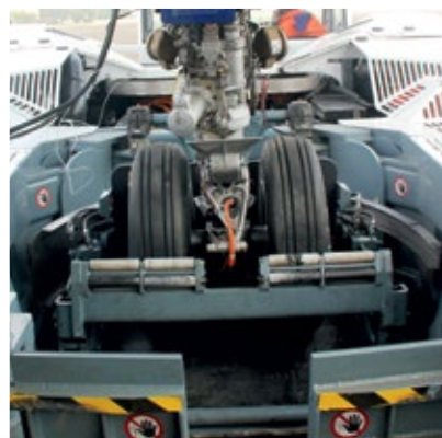
ABOVE At Frankfurt Airport, operators ready TaxiBot for narrow-body and, TOP , wide-body aircraft. BELOW A close-up of the mechanism on a cradle being tested on an A320.
